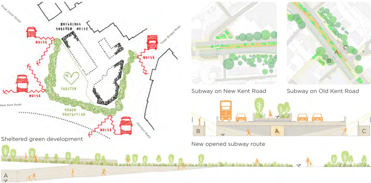
Proposal - Sheltered pedestrian spaces at ground/subway level A: NEW ROUTE FROM SUBWAY LEVEL TO PROVIDE DIRECT ACCESS TO THE FLYOVER WITHOUT CROSSING B: EXISTING SUBWAY, REMODELLED TO PROVIDE A SAFE PASSAGE THROUGH C: EXISTING SUBWAY, REMODELLED TO PROVIDE A SAFE PASSAGE THROUGH
