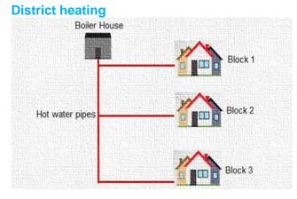
District heating properties are served from a main boiler house. These pump hot water into the radiators and cylinders in each property.
