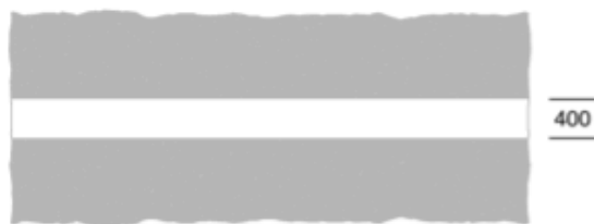
1002.1 Vehicular traffic must not proceed beyond the line when required to stop by the sign shown in diagram 601.1
